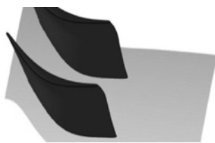
图 10 第二列静子叶片三维造型 Fig. 10 Three-dimensional geometry of the second stator
