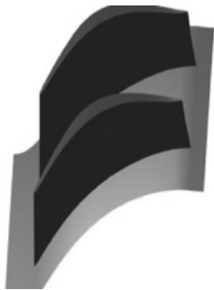
图 9 第二列转子叶片三维造型 Fig. 9 Three-dimensional geometry of the second rotor
